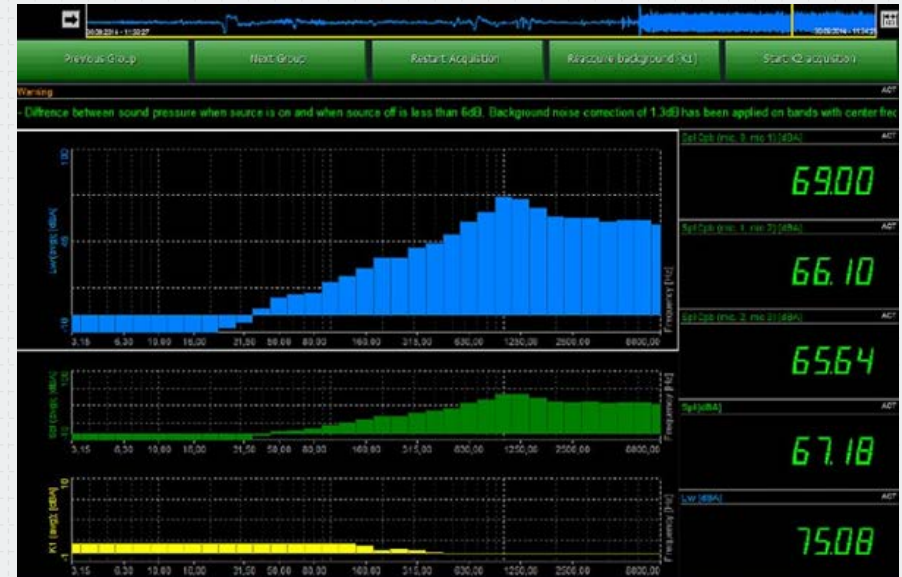
Figure 7. Sound Power measurement in Dewesoft software.
