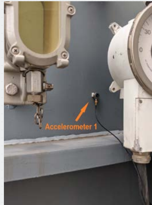
Figure 2. An accelerometer was used at two different positions on the reactor during the test - on the exchanger side and the HV output side.
