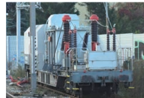
The High-Voltage Test Car from ÖBB-Infrastruktur AG checks the electrical infrastructure on the railway across Austria.
