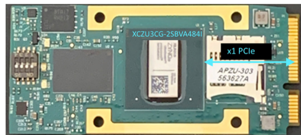
Figure 6: All AcroPacks include a x1 Gen1 PCIe link
