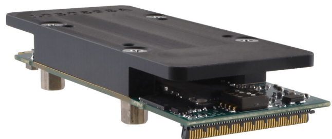
Figure 9: APZU with heat spreader
