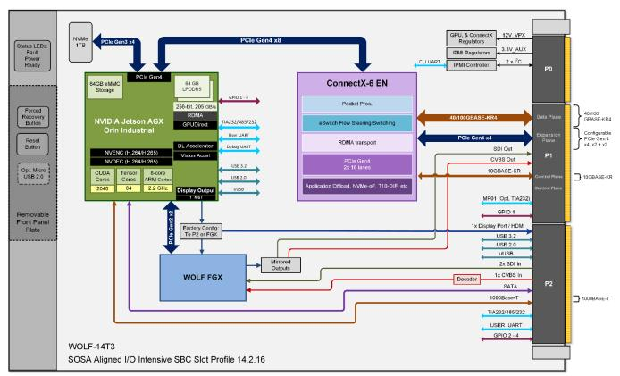
The following model provides two 10GBASE-KR, one 1000BASE-T and PCIe Gen4 up to 8 lanes.
