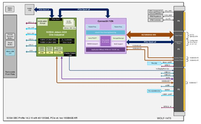
The following model provides two 10GBASE-KR, one 1000BASE-T and PCIe Gen4 x8 (configurable).
