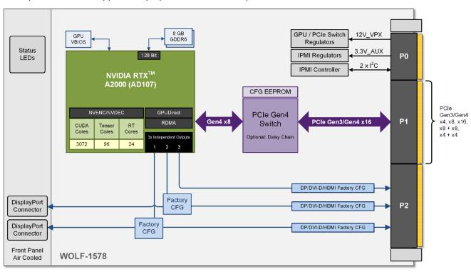
The SOSA Aligned HPC model supports slot profile 14.6.11 with PCIe supported on P1B.
