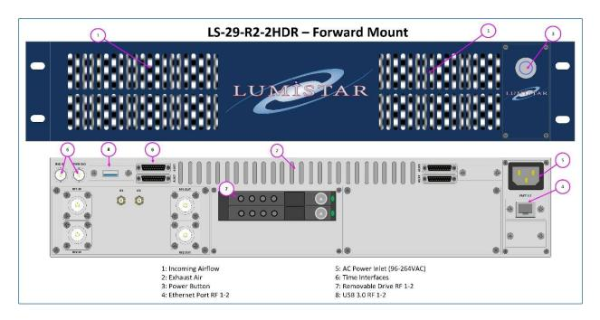
LS-29-R2 Series RF Recording/Playback System Two Channel / Enhanced Dynamic Range Version Front and Rear Panel Elevations
