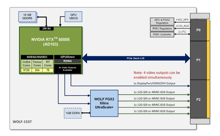
The Ada RTX 5000 GPU supports up to 4 video outputs, which can be routed to the WOLF FGX2 to be converted into SDI (up to 12G-SDI data rates) or ARINC 818 formats. Optionally one of the 4 video streams can be routed to the rear to be output as DP/HDMI/DVI. Additional DDR4 memory can be included if the video conversion requires an extra frame buffer.
