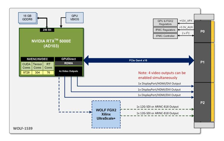
The Ada RTX 5000 GPU supports up to 4 video outputs. Three of those outputs are routed directly to the P2 connector. One is routed to the P2 pinout assignment used for SOSA Aligned SBCs for ease of integration, and also to provide compatibility with the cables typically used in lab settings when a backplane may not be available (e.g. Meritec cables). Note that in order to accommodate the SBC video pin mapping this product is not pin compatible with WOLF-1538.
