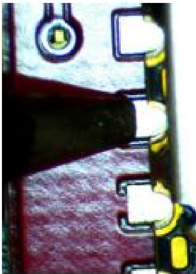
(a) Recommended Soldering Tip
