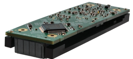
QMC Module shown with attached heatsink. Heatsink optionally sold with QMC Modules.
